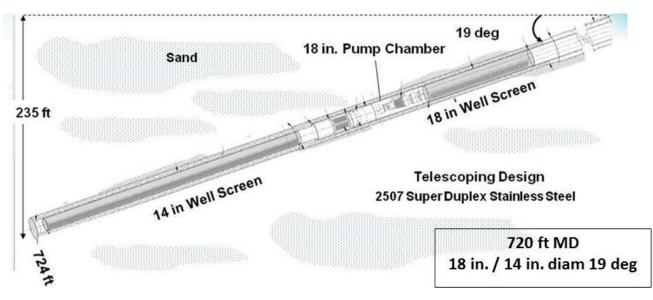
Figure 5. MPWSP Test Slant Well Showing Telescoping Design
