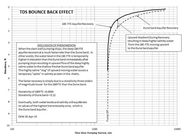
Figure 7 MPWSP Test Slant Well Showing Water Quality Variation During Recovery
